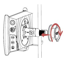
2) Position the bracket on the vertical tube and tighten the knob until the assembly is immobilised.
