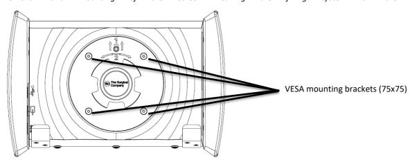
Next, attach the Screeni to the VESA mounting bracket (not supplied) using four M4 x 10 mm screws (not supplied).
