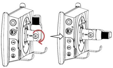
1) Unfold the quick-connect bracket.
